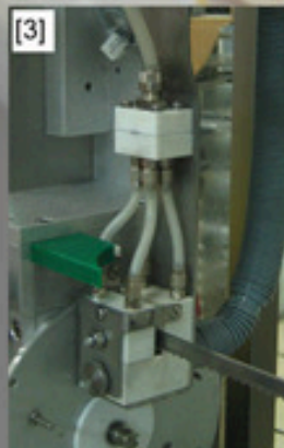
[2] + [3] cutter cleaning system with steam/suction combination for automatic cutter cleaning between the timed sequences of cutting
